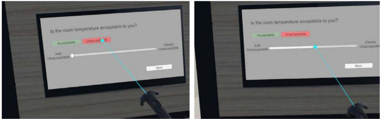
Figure 4: Thermal acceptability question. Left: Pressing 'unacceptable' using the controller pointer. Right: Moving unacceptable slider using the controller pointer to determine the degree of unacceptability.
