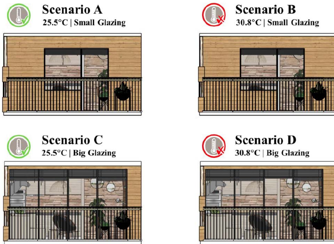
Figure 1: The four investigated scenarios. Two different operative temperatures combined with two different glazing sizes.
